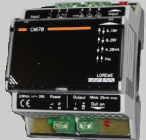
The converter CMi70 allows, from a standard analog signal (4 .. 20 mA, 0 ..10V, ....), to generate a logic signal with a 0 to 100% variable duty cycle to drive power units or static relays used for regulation of heating element.
