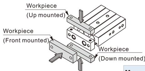
**Be mounted cylinder from four directions**
