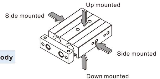
**Magnetic switch slots around the cylinder body**
