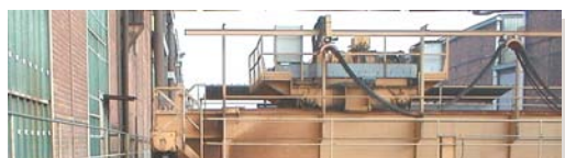
← 3 cranes operating outdoor on a 456 metres system, comprising 3 x 1250A Phase and 1 x 800A Earth conductor.
