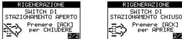
With the switch closed, the regeneration can also be started with a press of the ACK\_BUTTON:
