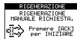
The Stationary regeneration can be interrupted by deactivating the parking switch, turning the engine off, or disabling the regeneration just like for the Reset regeneration.
