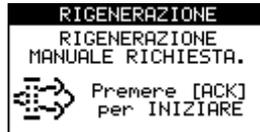
With regeneration in progress, the REGENERATION TIMER is displayed, indicating the time remaining to the end of the regeneration, sent by the engine ECU
