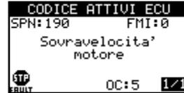
In this case, the icon on the lower left corner indicates the status of the RED STOP and AMBER WARNING signals sent by the DM1 command. Fault translations are:
