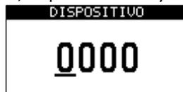
One digit is entered at a time; use the LEFT\_BUTTON and RIGHT\_BUTTON to move the cursor, and the UP\_BUTTON and DOWN\_BUTTON to change the digit. To test, use the ACK\_BUTTON until the result appears:
