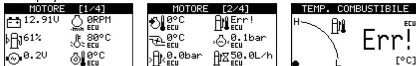
The instrument can be disabled and greyed out even if the ECU returns a correct value.
